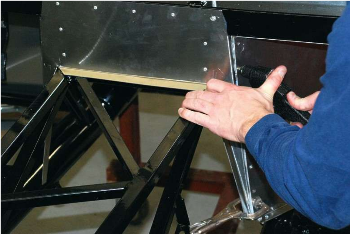
Silicone and rivet the panel to the front tunnel "A" and the footbox top.
