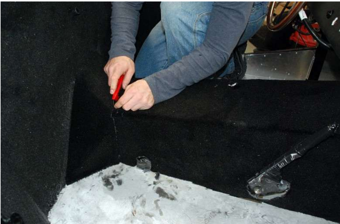
The tunnel rear section is slightly oversized to make sure it can cover small variances in the way the other pieces lay down. Trim it for a perfect fit then glue it in place.
