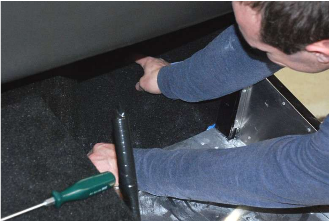
Fit and glue the lower floor sections.
