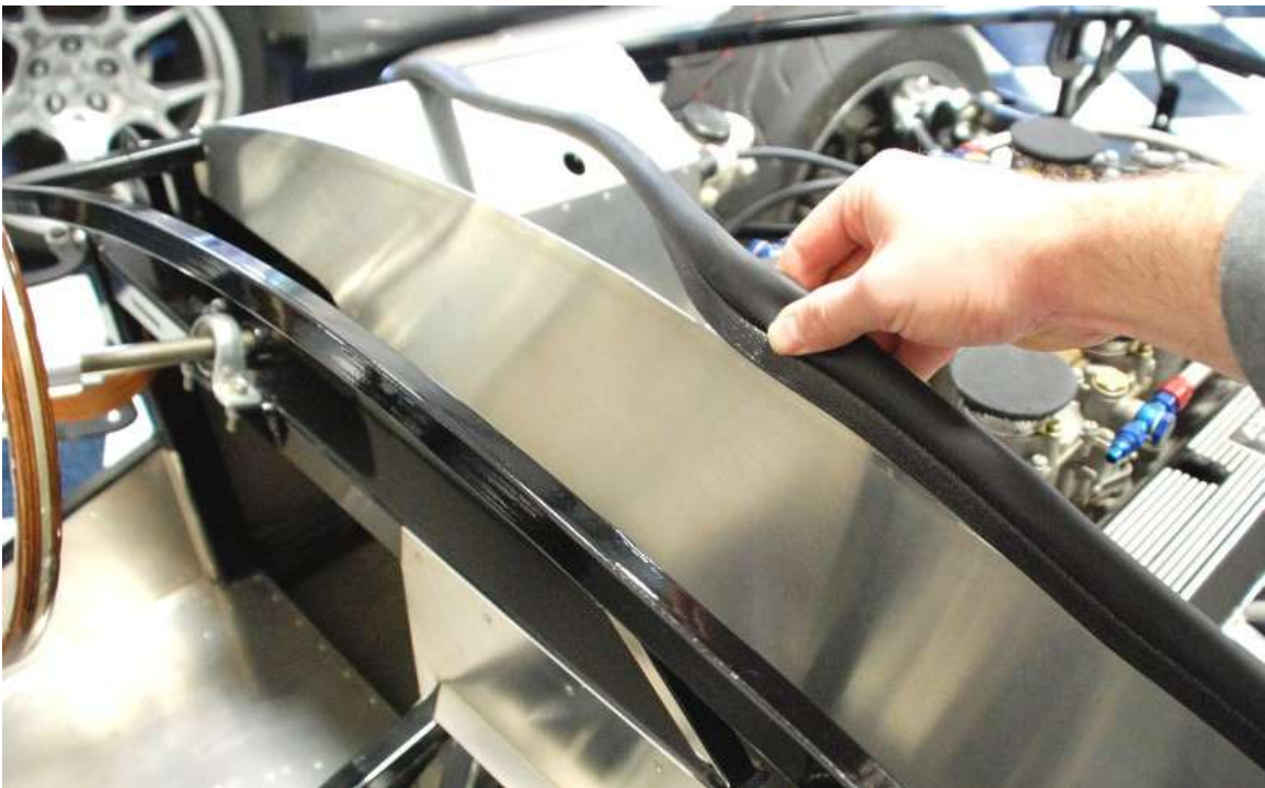
The push-on weather strip goes across the top of the firewall
