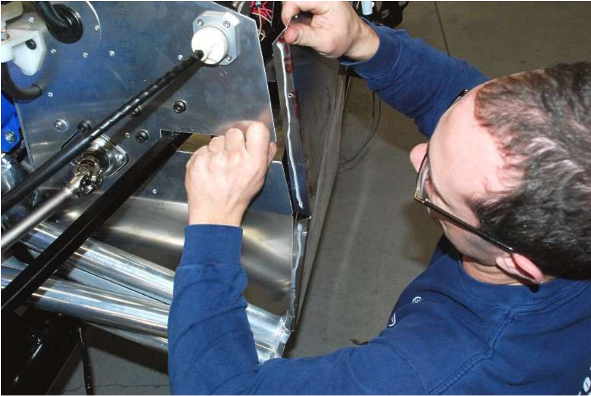
Silicone and install the driver's side footbox outer wall. The front flanges tuck in behind the footbox front panel.
