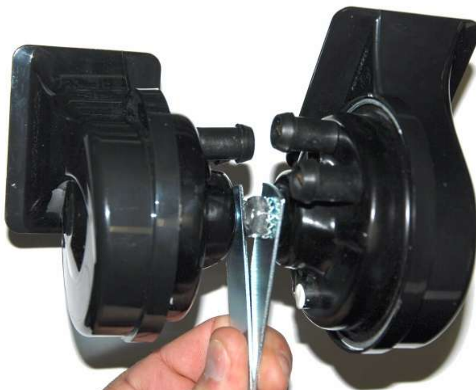
Holding the horns, the connectors should be spaced so that the wires will not hit each other.
