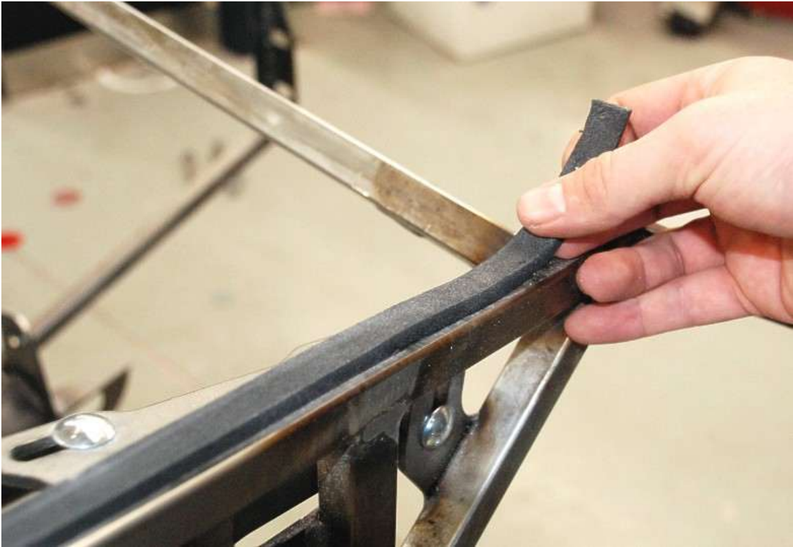
The rectangular adhesive backed weatherstrip runs along the top of the chassis tubes on either side of the hood opening and the top of the curved trunk hoop.
