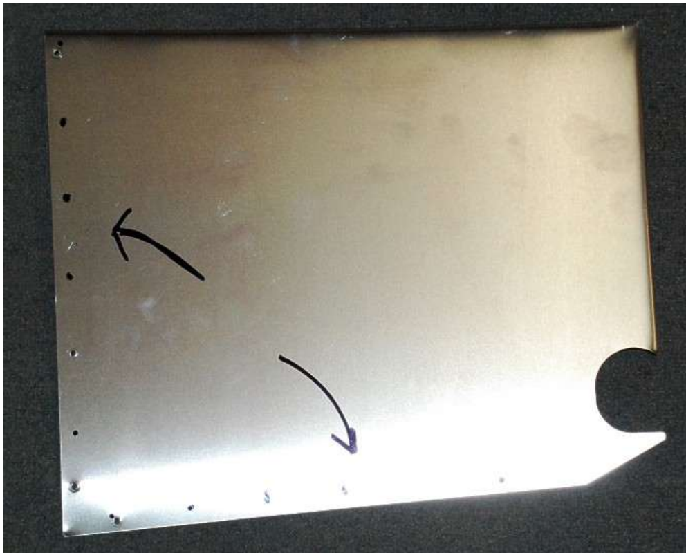
Mark the holes in the passenger footbox front panel upper and outer edges but do not drill yet.
