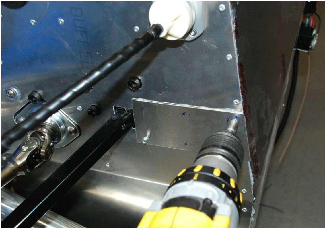
Silicone and install the front patch panel.
