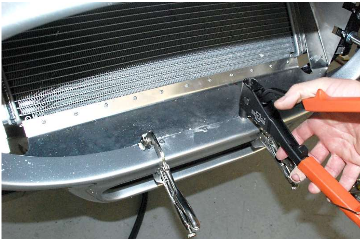
Silicone and rivet the aluminum to the nose lip using three \frac{3}{16} " rivets.
