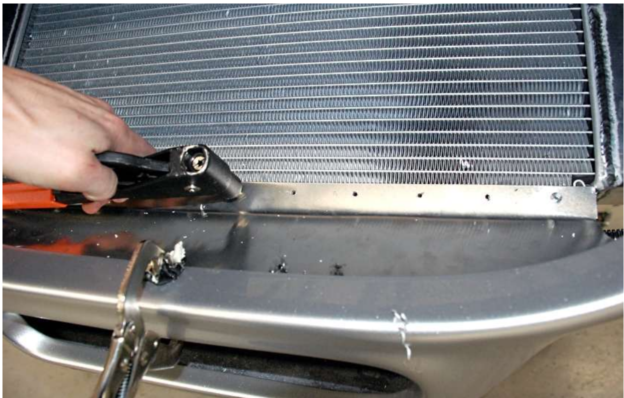
Drill, silicone and rivet the radiator floor aluminum to the bottom radiator lip.
