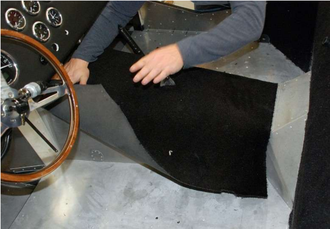
Glues down the tunnel top.
