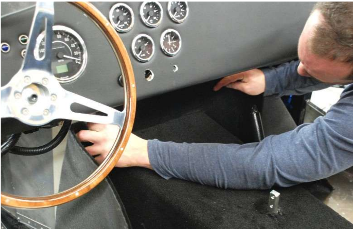
Fit and glue the tunnel/firewall section of carpet.
